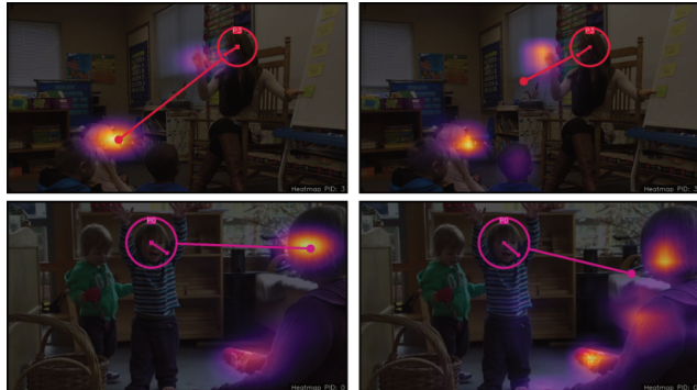
Figure 6. Comparison of Heatmap ( i.e. left) and 2D Point regression model ( i.e. right) models. The heatmap on the right is obtained by computing the attention weights ( i.e. last encoder layer) of the person’s gaze token with the image tokens.
