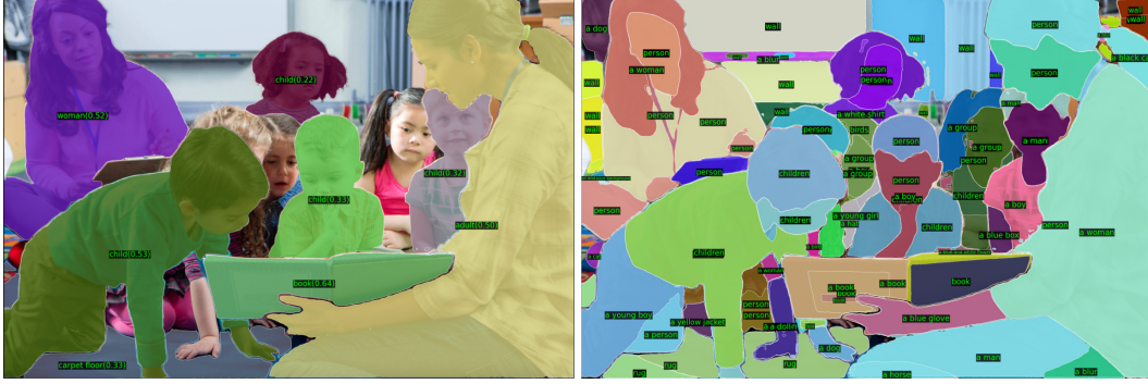
Figure 9: Comparison of the outputs of the segmentation methods. Left: RAM-Grounded SAM. Right: Semantic-Segment-Anything.
