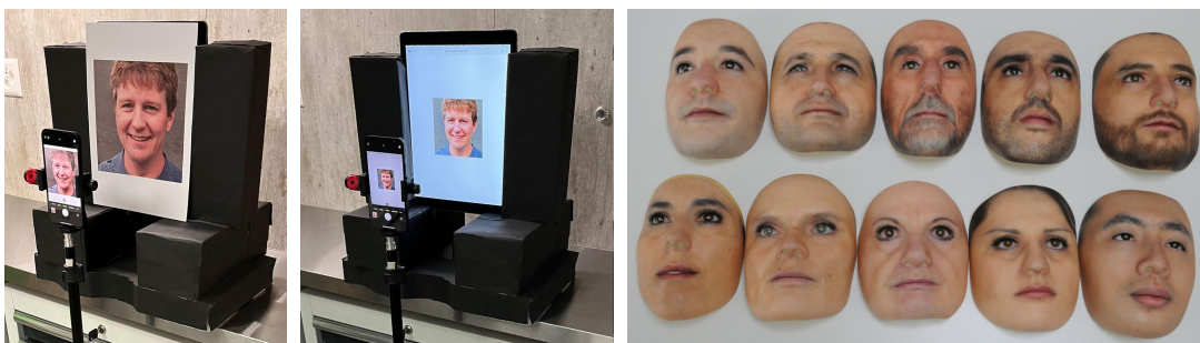
(a) A print attack, from [7] (b) A replay attack, from [7] (c) Various 3D face masks. With permission from Sébastien Marcel.
