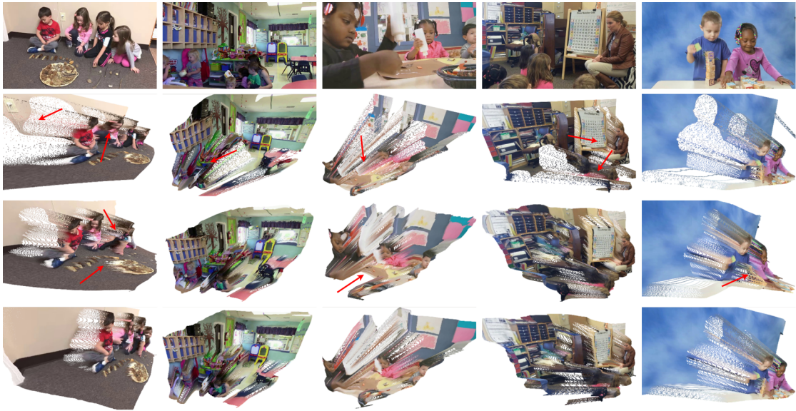
Figure 5.7: Comparison of point clouds generated using the depth maps from Ranftl et al. (Ranftl et al., 2020) (row 2), Wei et al. (Yin et al., 2021) (row 3) and Patakin et al. (Patakin et al., 2022) (row 4) on ChildPlay images. The point clouds generated using Patakin et al. appear to best preserve the geometry of the scene.
