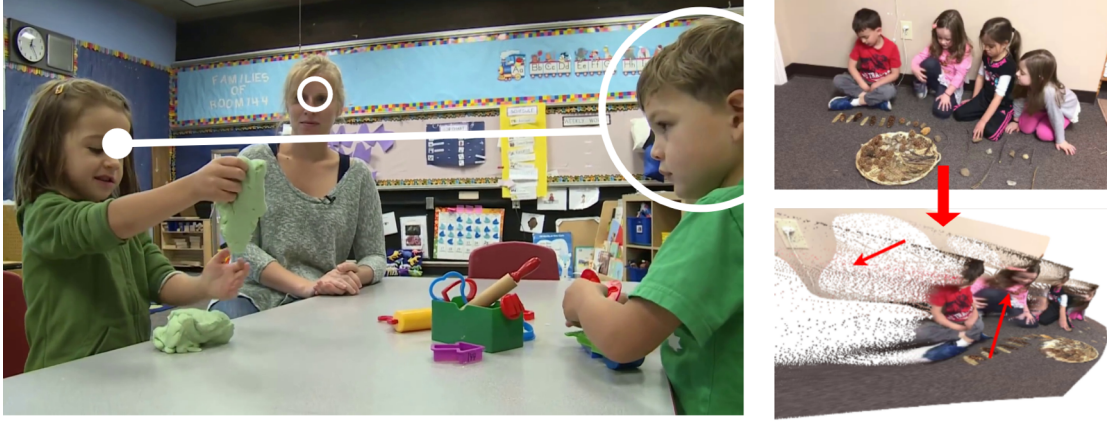
Figure 5.4: Depth is crucial for gaze following, as it enables reasoning about the 3D structure of the scene and helps rule out salient objects that lie along the 2D line of sight but are not visible in 3D (left). However, typical methods rely on disparity maps (e.g. (Ranftl et al., 2020)), which often produce distorted point clouds (right) and thus limit 3D reasoning.
