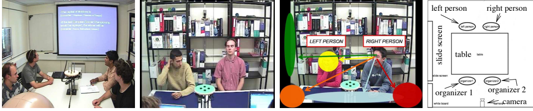
Figure 2.1: Early approaches for VFOA estimation relied on specialized hardware, such as calibrated camera setups or pre-specified scene layouts. In this example from Ba and Odobez (2008), both object and person locations are predefined within the environment.
