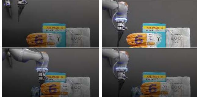
Figure 9.6.: Top left image shows the initial state of the experiment. Top right illustrates the plate gripper pose after going down. Bottom left shows the end of the pushing movement, where the gripper is in contact with the object. Bottom right shows the robot after coming back to the previous pose. These images were prepared by Ocado Technology.
