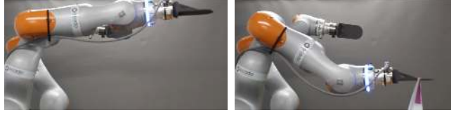
Figure 9.4.: Left: the start configuration of the robot, showing the desired pose of the plate gripper. Right: the result of the movement after attaching the item with 4.6kg to the gripper. These images were prepared by Ocado Technology.
