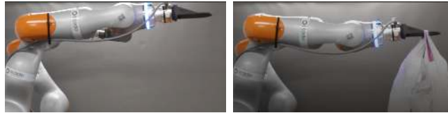
Figure 9.2.: Left: the start configuration of the robot, showing the desired pose of the plate gripper. Right: the result of the movement after attaching the item with 0.633kg to the gripper. These images were prepared by Ocado Technology.
