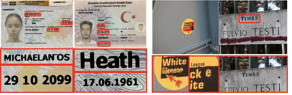
Fig 2: FantasyID [15] and OSTF [26] Two different templates from our proposed, FantasyID (left) and OSTF (right) dataset. The red box show the manipulated regions and their corresponding zoomed-in image. (Left) Altered text mostly show jagged edges due to inconsistent blending with the background. (Right) Zoomed-in view of the tampered region where some of the manipulation artifacts are visible. Such regions occupy small area of the full image making it a challenging detection task.
