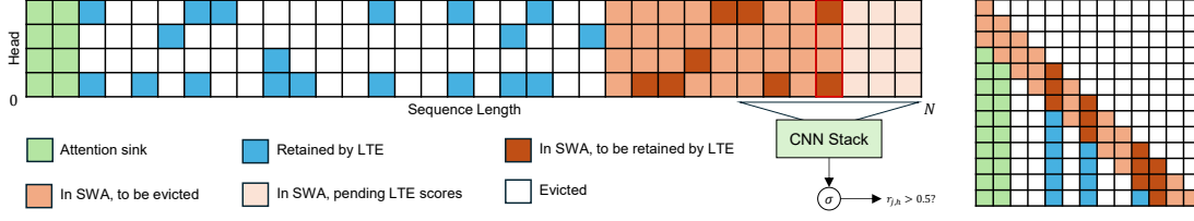
Figure 6.1: Left: Illustration of our eviction scheme, combining LTE, an attention sink (size s = 2 ), and SWA ( w = 12 ), with 4 KV heads. A CNN stack predicts a per-token, per-head retention score r_{j,h} when its receptive field is fully covered by the SWA window, which determines whether a KV pair is evicted once it leaves the window. With recent KVs cached by SWA, the CNN can read short-range past and future context. Right: The resulting per-head A-plus-column sparsity pattern; colored tiles denote tokens selected at each step.
