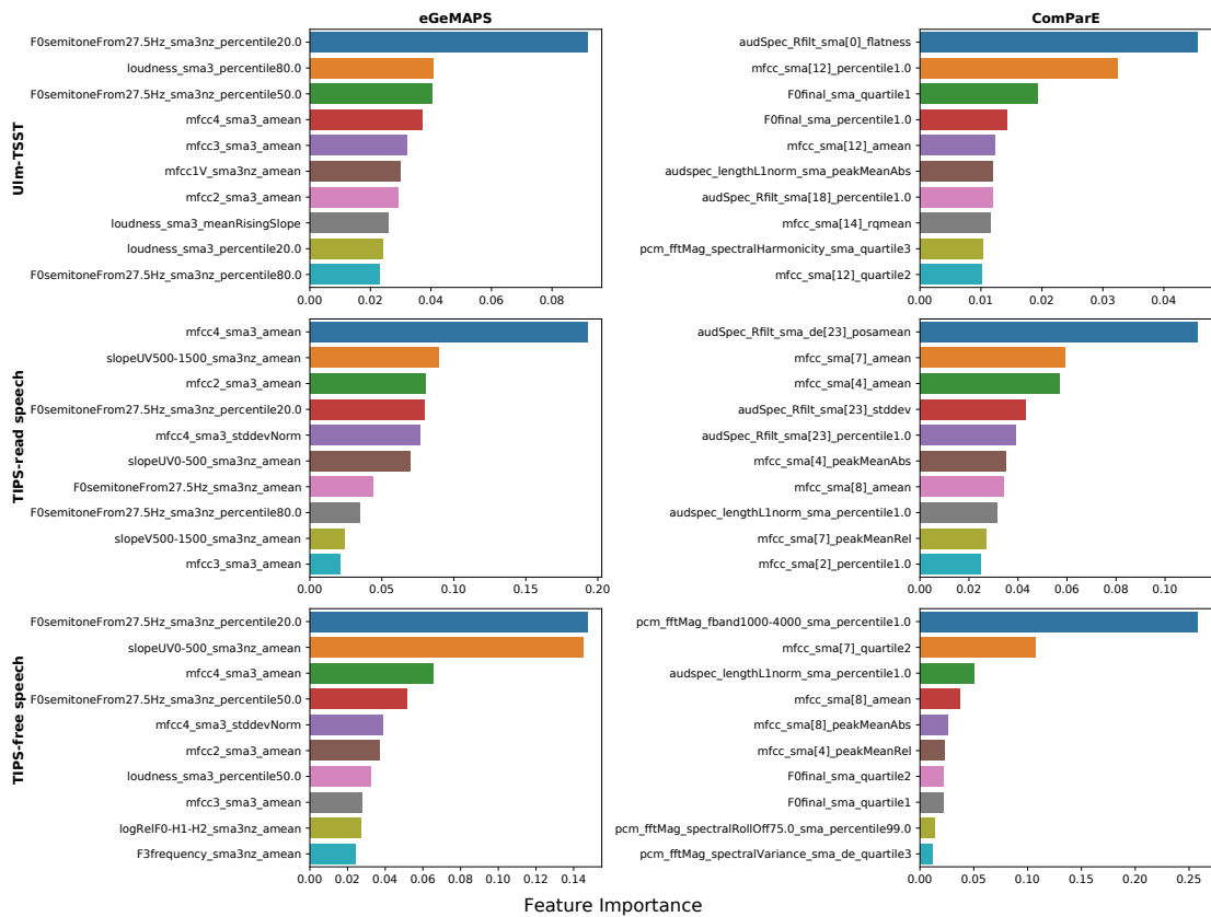
Figure 6.8 – Feature importance showing top 10 acoustic features for BPM extracted from both openSMILE feature sets, eGeMAPS and ComParE for the three data subsets. The feature names are denoted as LLD_filtering_functional
