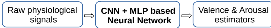
Figure 4.8 – Proposed pipeline for end-to-end system to estimate valence and arousal from raw physiological signals.
