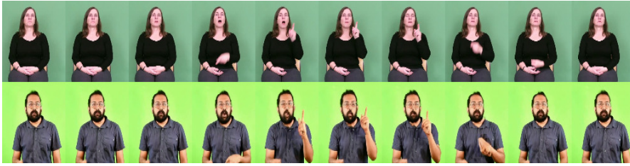
Figure 5.4 – First row shows the sequence of frames in the reference video for the sign "ABER", the second row shows the corresponding frames generated by the GAN.
