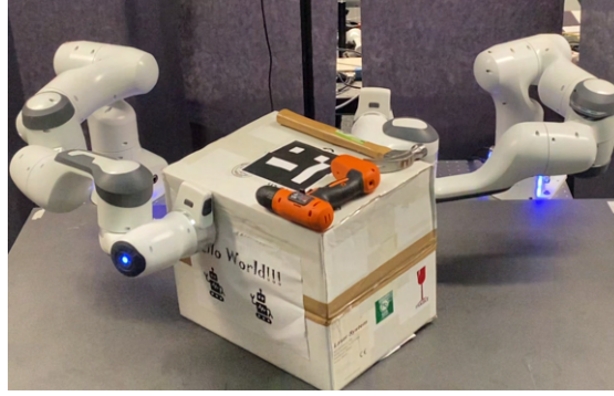
Figure 4.16: Experimental setup with mass perturbation. A 1.2 kg external mass is introduced to evaluate the robustness of TTTS against model mismatch between the real world and the Genesis simulation.
