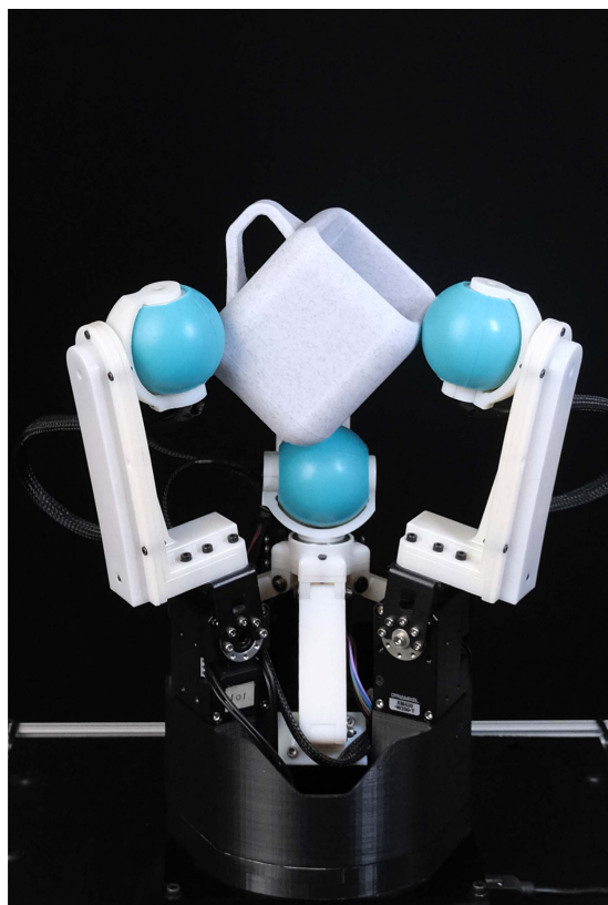
Fig. 1. Prototype of the Roller Grasper V3 holding a 3D-printed mug.
