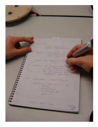
Figure 5: Capture of handwritten notes by using Logitech pens.
