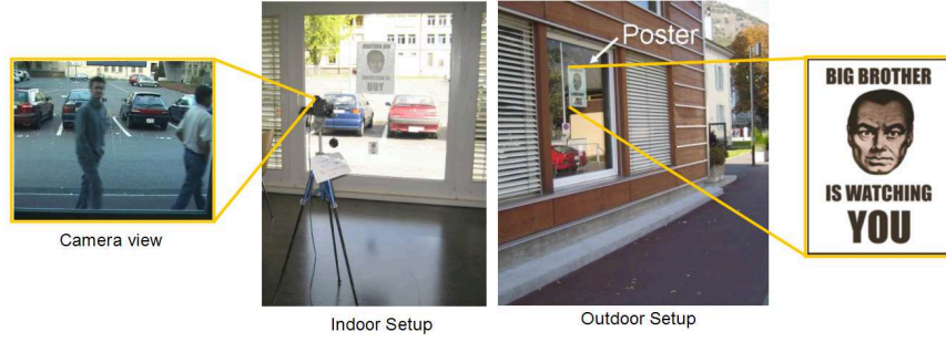
Figure 6.6: Experimental Setup . (Left) Inside the building, a camera is placed so that it is facing out a window. The view from the camera can be seen in the insert. (Right) Outside, the advertisement in the window is noticeable to people walking along the footpath. The fake advertisement poster can be seen in the insert.
