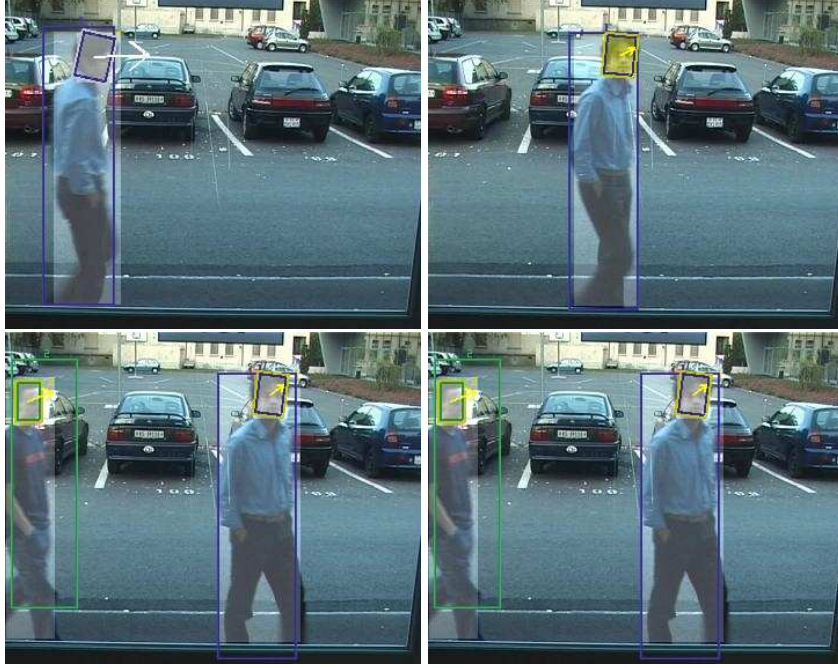
Figure 1.4: Moving people's VFOA recognition. People passing by a glass windows are tracked, their head poses estimated. A model using as observation head locations and poses is used to estimate whether or not they are focusing an advertisement posted on the glass windows.
