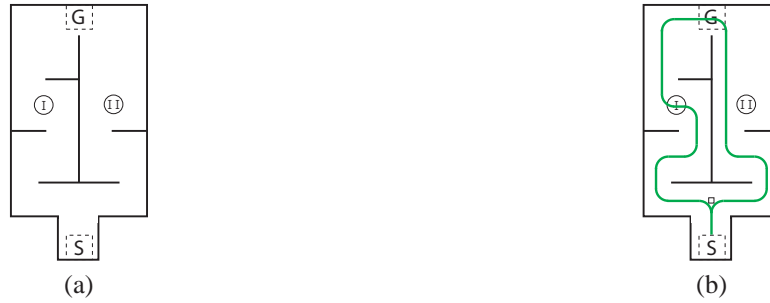
Figure 9: (a) Experimental environment for experiment C: two possible ways for going to a same goal location. (b) Graphical representation of the paths. The square \square indicates where the user provided an error signal.
