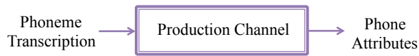
Fig. 2. Phone attribute encoding: Speech production channel transmits the source phoneme information through production of the target phone attributes.
