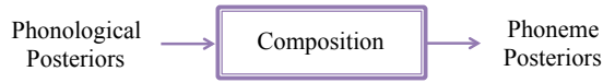
Fig. 3. Phoneme decoding: Phoneme perception operates on the basis of merging evidences on phone attributes composition.
